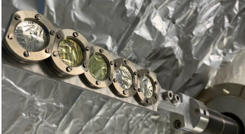
FIGURE 5.11: The degrader ladder with five different foils mounted. Each foil is either 100 nm or 200 nm of Parylene N. For this configuration, the effective thickness of each degrading stack is: 400 nm ( 2 \times 200 nm), 300 nm ( 200 nm + 100 nm), 200 nm, 200 nm, 100 nm. Picture taken from [56].
