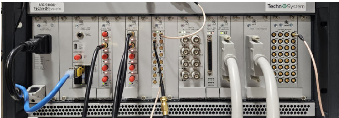
FIGURE 5.17: One of the Sinara crates used at AEGIS. It consists of 10 modules. From left: power module, Kasli carrier, two DDS-based frequency synthesisers ("Urukul"), 16-channel digital I/O unit, 8-channel analogue-to-digital converter ("Sampler"), 32-channel digital-to-analogue converter ("Fastino"), 32-channel HV amplifier, HD86-IDC adapter, IDC-MCX adapter.
